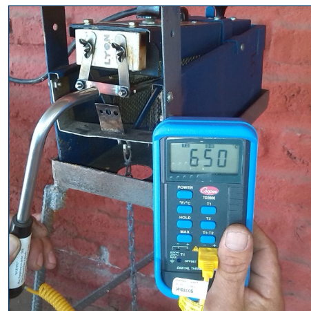
Pyrometer indicating proper blade temperature of 650°C.
